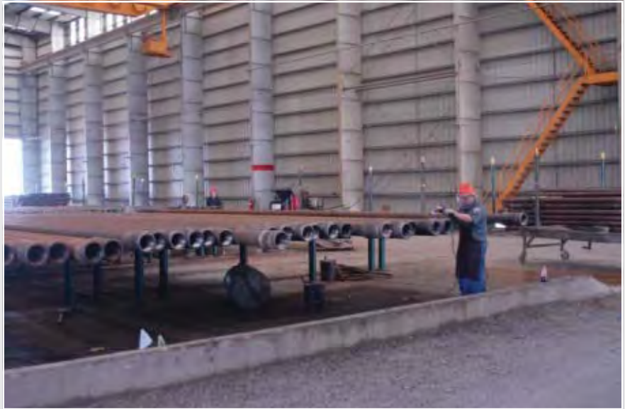
(Above) At the Smith Services facility in C-Port II, drill pipe and other tubulars arrive straight from the rig to be cleaned, inspected, and, if necessary, repaired before returning to operation. (Below) With the portable load test unit, Halo can simulate an actual lift at a client’s facility.
